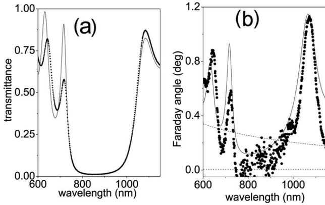
FIG. 1. (a) The experimental spectra (circles) of the transmission and (b) the Faraday rotation angle  $\theta_{pc}$  of the 5.5 pair MPC measured at the normal incidence and corresponding numerical approximation by the  $4 \times 4$  matrix method (lines). Dashed line is the spectrum of the Faraday rotation angle  $\theta_0$  in homogeneous Bi:YIG slab of the same thickness as the total thickness of Bi:YIG in MPC.
