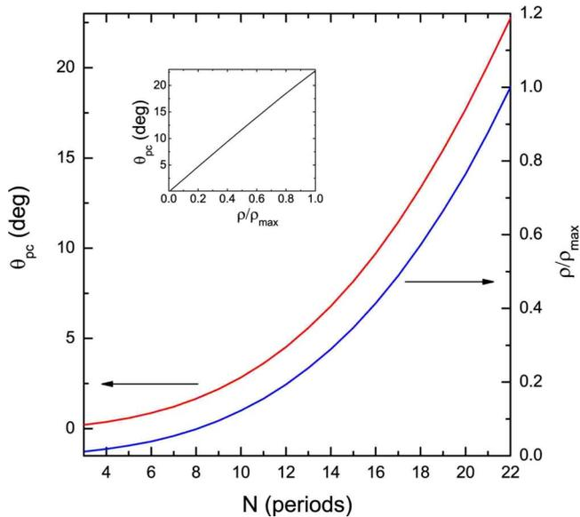
FIG. 4. (Color online) Size dependence of the normalized optical field  $|E(N)|^2$  is shown by blue (dark gray) line and the Faraday rotation angle  $\theta_{pc}(N)$  is shown by red (light gray) line for the long-wavelength band edge of finite MPCs. Inset shows corresponding linear dependence of  $\theta_{pc}$  on  $|E|^2$ .
