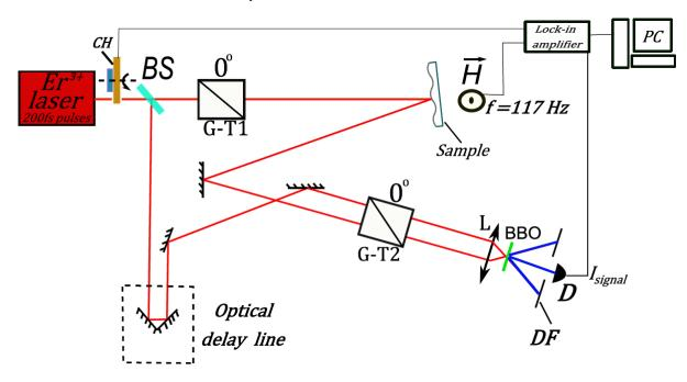
Fig.1. Experimental setup for measurements of second-order correlation functions. CH is a mechanical chopper, BS is a beam splitter, G-T1 and G-T2 are Glan-Taylor polarizers, L is a focusing lens, BBO is a nonlinear optical crystal, D is a detector, H denotes the external AC magnetic field, DF is an aperture.
