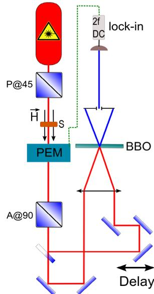
Fig. 1. Experimental setup scheme. P - polarizer, A – analyzer, S - sample, H - magnetic field, PEM - photoelastic modulator.
