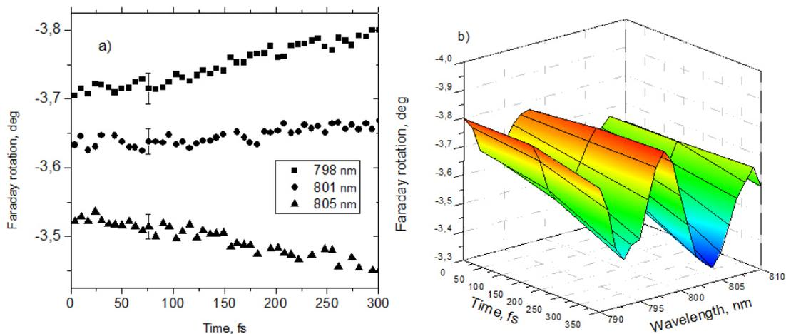
Fig. 2.a) Time dependence of Faraday rotation in thin magnetic film. Squares correspond to 798 nm wavelength of source and maximum of transmittance spectrum, triangles correspond to 805 nm wavelength and of transmittance spectrum and circles correspond to 801 nm and intermediate case. b) Spectral characteristics of time dependence of Faraday effect in thin magnetic film.
