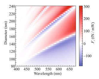
**Fig. 3.** (Color online) Dependence of the normal component of the force acting on a silicon particle in the field of a Bloch surface wave on the light wavelength and particle diameter. The gap between the waveguide surface and the particle is fixed and equal to h = 30 nm; the force values are normalized to the optical power in the surface wave mode.
