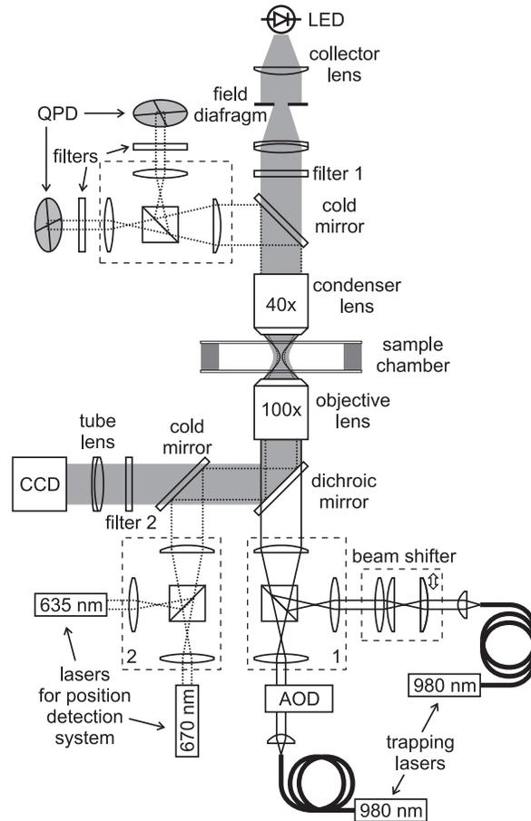
Figure 1. Sketch of the experimental setup: double-trap optical tweezers for RBC elastic properties monitoring. 1, 2 — systems for the conjugation and expansion of the laser beams.
