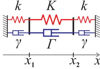
Figure 4. Phenomenological mechanical model of the trapped RBC,  $k$  is the trap stiffness,  $K$  is the RBC elastic coefficient,  $\gamma$  and  $\Gamma$  are effective viscous coefficients of the trapped system.
