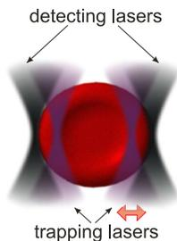
Figure 2. Single erythrocyte trapped by two infrared trapping lasers. One of the trapping lasers position is oscillating with an amplitude of 100 nm in the frequency range from 50 Hz to 1 kHz which is schematically shown by the arrow. Two extra lasers which are focused on the RBC edges are used for the RBC edges positions detection.
